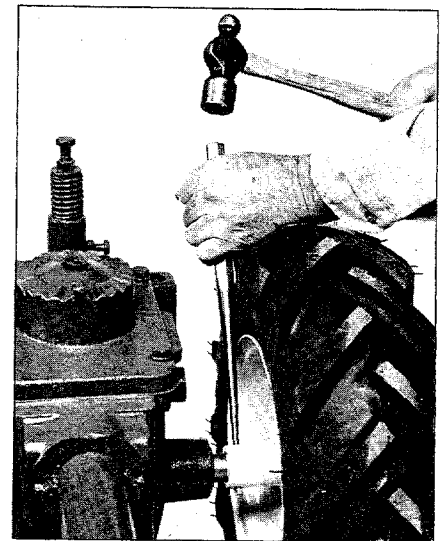
Photo 5-34: Drive roll pin out to remove wheel. Grease wheel shaft before replacing wheel.
